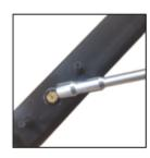
STEP 12: Loosen the orifices (wrench 7) and replace them with the orifices for Natural Gas.and air inlets.
