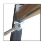
STEP 10: Unscrew the M5 bolts to loosen the burner tube from the manifold tube.
