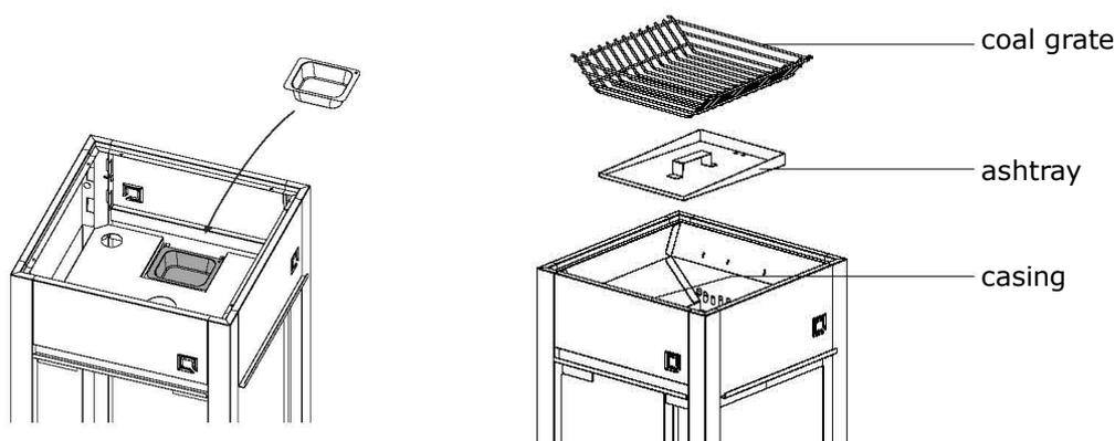
We recommend cleaning the parts of the oneQ glow after each use. Empty the ashtray after each use. Check all places where oil, grease or food residue may accumulate, then all components remain in optimal condition.
